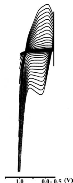
Fig. 3. Cyclic voltammogram of PStPy in the presence of Py at a scan rate of 500 mV s -1 .
